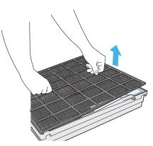
4. Remove the white Medium Filter from the black frame to discard the plastic wrapping. Return the filter to its frame.
