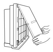
2. Remove the fillter case by grasping the handles on either side and pulling forward. Lay the filter case on a flat surface.
