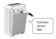
Step 3 Place activated carbon filter screen as shown in the figure. Grasp the activated carbon filter in the direction of the arrow and put the unpacked activated carbon filter back into the appliance with the tag pointing towards you.
