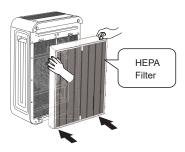
Step 4 Place the HEPA filter as shown in the figure. Grasp the high-efficiency HEPA filter as shown by the arrow and put the unpacked high-efficiency HEPA filter back into the appliance with the tag pointing towards you.
