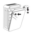
Step 5 Place the bottom of the pre-filter frame into the slots on the bottom of the appliance and press the top towards the appliance.
