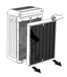
Step 3 Pull the tag of the HEPA filter to remove the filter from the air purifier
