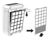
Step 2 First press the clasps of the pre-filter down, releasing the frame. Then pull the pre-filter towards you, and finally lift the pre-filter upwards.
