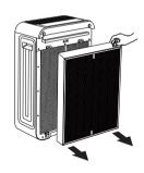
Step 3 Pull the tag of the HEPA filter to remove the filter from the air purifier
