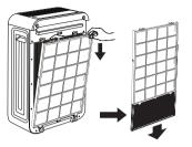
Step 2 First press the clasps of the pre-filter down, releasing the frame. Then pull the pre-filter towards you, and finally lift the pre-filter upwards.
