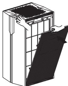
Step 6 Place the filter cover on the unit once all the filters have been installed. Repeat steps 1 - 6 on opposite side.
