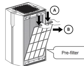
Step 2 Press down on the Pre-filter tabs (A) and pull outwards to remove (B). Gently remove the filter and PRO-Cell Catalyst from the appliance and remove the packaging.
