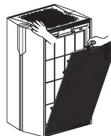
Step1 Grasp the handle on the panel with one hand and gently pull outward to remove.
