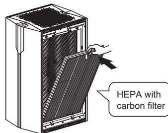
Step 4 Next, place the unpackaged HEPA with carbon filter back into the appliance with the tag pointing outwards.
