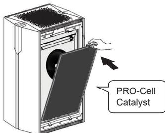
Step 3 Gently place the PRO- Cell Catalyst (metal honeycomb) in the innermost position closest to the UVC lamp as shown in the figure with the tag pointing outwards.
