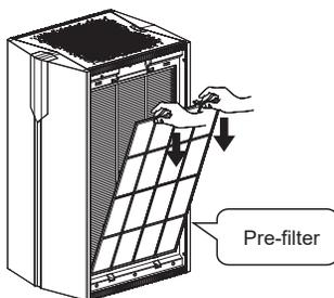
Step 5 Place the Pre-filter frame into the slots on the bottom of the appliance and press the top towards the appliance until the clasps click.
