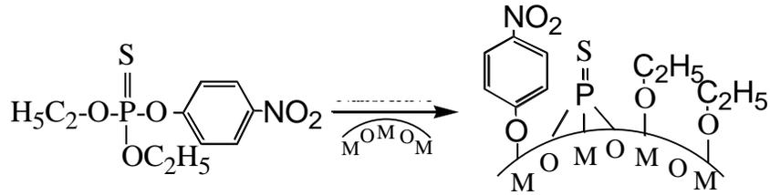
Upon exposure of parathion to the EnviroKlenz material (“MOMOM” metal oxide surface), chemical bonds between the phosphorus and oxygen are broken and the fragments are adsorbed on the surface of the EnviroKlenz product.
