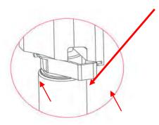
6> Load the new H13 filter: Place the new H13 filter on the locking tray. (Note: It is necessary to put filter with the pull tab towards to the user)
