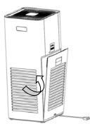
2> To unlock the filter lock: Hold the filter lock block and pull it out. When pulled out, the filter unlocks and descends.
