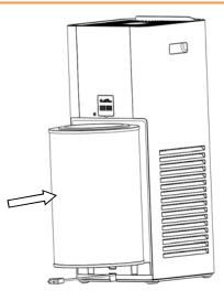
7> Lock the H13 filter: push the filter locking block inward as show below
