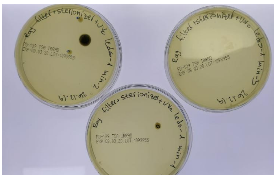
Figure 13: incubation results of the Ray filter+ Sterionizer+ UVc LEDs plates on December 31 st ,2019
