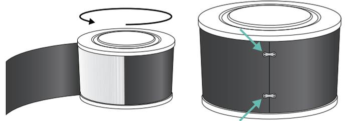
4. Slide the HEPA Cartridge with new Carbon Prefilter back in the center of the unit.
