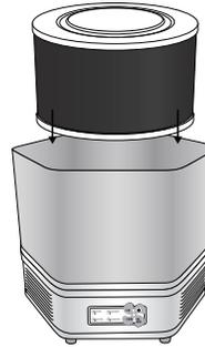
5. Gently press down on the HEPA Cartridge and turn clockwise until it locks into place.
