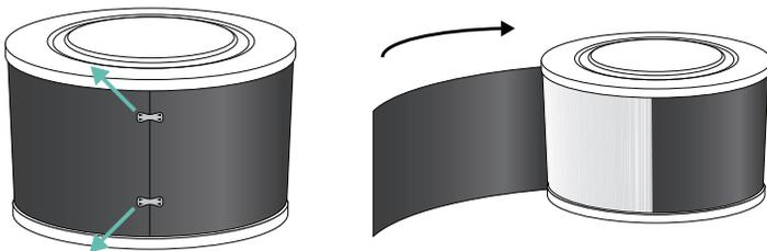
2. Remove plastic packaging from the new Carbon Prefilter.
