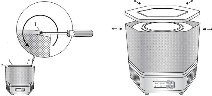
3. Bracing the unit so it does not move, gently press down on the HEPA Cartridge and turn counterclockwise until it unlocks, then lift the HEPA Cartridge out of the Air Filtration System.
