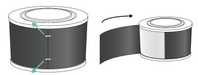
2. Remove plastic packaging from the new Carbon Prefilter.
