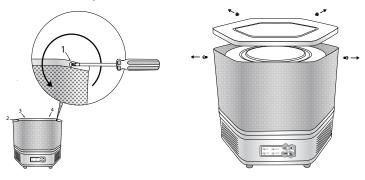
3. Bracing the unit so it does not move, gently press down on the HEPA Cartridge and turn counterclockwise until it unlocks, then lift the HEPA Cartridge out of the Air Filtration System.
