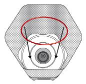
3. Place the V.O.C. Canister inside the Air Filtration System, centered on the intake hole to the motor section. The end of the V.O.C. Canister without the screws is placed down.
