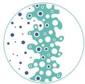
Carbon is to V.O.C.'s as what a sponge is to water. When V.O.C.'s come into contact with the carbon filter, they become trapped in tiny capillary passages on the surface of the carbon. This process can continue until all the passages are filled, much like saturating a sponge. The larger the surface area of the carbon, the more V.O.C.'s it can hold.
