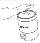
STEP 3 Remove lid by pulling slightly on cover.
