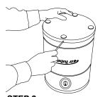
**STEP 2** Using a #2 Philips screw driver, remove all 4 screws.
