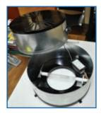
**STEP 3**Carefully, remove halfway the blower compartment, enough to clear the UV bulb.
