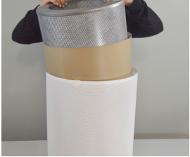
7. Insert the carbon filter into the top of the funnel and allow to slide in.
