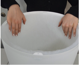
4. Roll new prefilter around the sides of the purifier.
