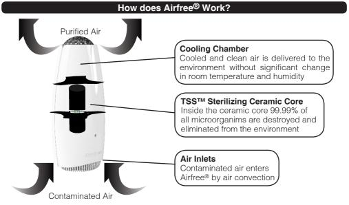
Regardless of how hazardous a virus, fungus or bacteria might be they are fully destroyed by the powerful heat inside the TSS™ ceramic core mini ducts. The heat inside the ceramic core forces sterilized air up to the heat exchanger causing air convection, which generates negative pressure underneath the ceramic core, so contaminated air is "sucked" in at Airfree<sup>®</sup> bottom air inlets in a continuous, silent, and efficient air flow.
