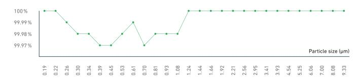
Filter media TFH 91-03: Cleaning performance measured at 100  $\text{m}^3\text{/h}$  as per DIN 71460-1 (AC Fine particle size 0.19–9.33  $\mu\text{m}$ )
