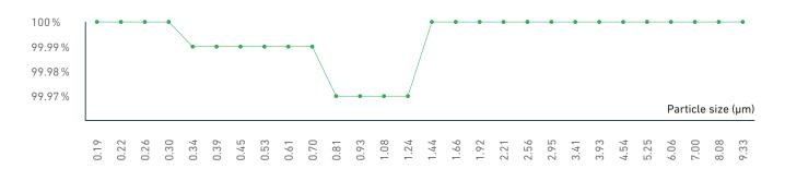
Filter media TFH 91-03: Cleaning performance measured at 124 m $^3$ /h as per DIN 71460-1 (AC Fine particle size 0.19–9.33  $\mu$ m)
