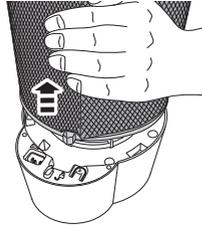
Unlock the filter cartridge at the locking component (A) and remove.
