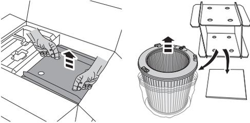
Lift the filter cartridge out of the box, unpack it and remove the protective film.
