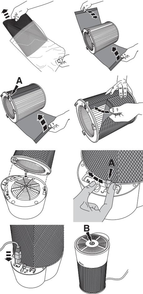
Take the textile cover (only IDEAL AP40 PRO) out of the protective film, place it around the filter cartridge and close it at the back (locking component **A**).
