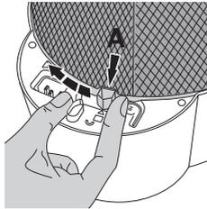
Insert the filter cartridge with the three snap-fit tabs into the three recesses provided for this and lock it at the locking component (**A**)
