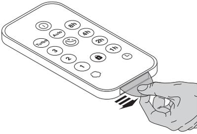
The remote control has a pre-installed lithium battery CR2025. **Remove the protective flap** to activate the remote control battery.
