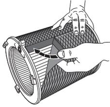
Put the textile cover (only IDEAL AP40 PRO) back on the filter cartridge and close it at the back (locking component **A**).
