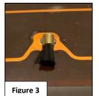
NPBI electrodes, or "needles," are made from carbon fiber (see Figure 3), titanium, silver, gold, stainless, or any other corrosion resistant, conductive material. As you can see from Figure 3, the electrodes are attached to the flexible circuit and there is no dielectric.
