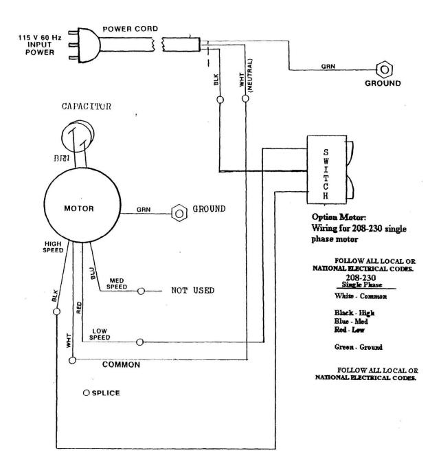
NOTE: For 277 voltage, wiring is the same as 208-230 single phase.
