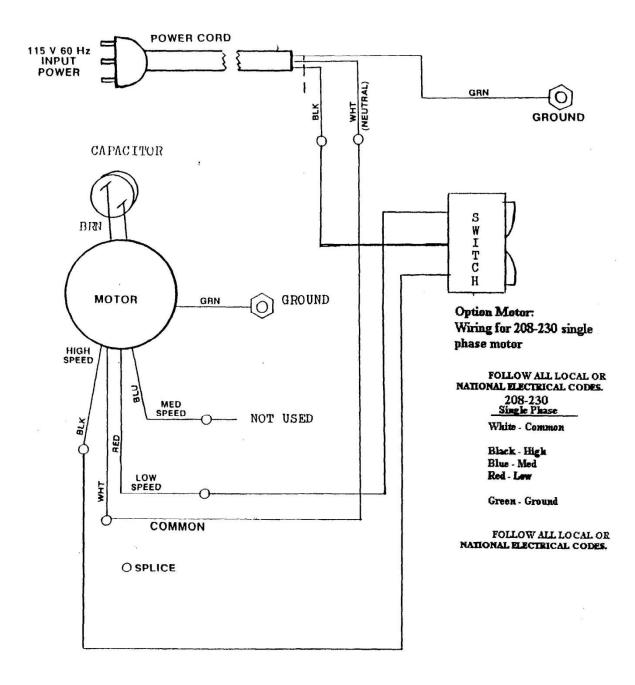
NOTE: For 277 voltage, wiring is the same as 208-230 single phase.
