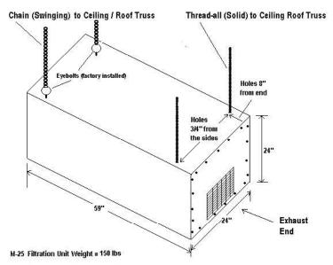
Electrical: 115VAC Single Phase with 12' power cord drawing 10.2 Amps
